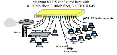
A diagram of the installation is shown here.
